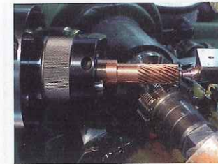
Helical gear electrodes must be generated on a gear hobber for perfect form. Just leaning the wire is not good enough!
