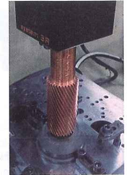
Helical gear cavities are still burned utilizing C-Axis in Sinker EDM.
