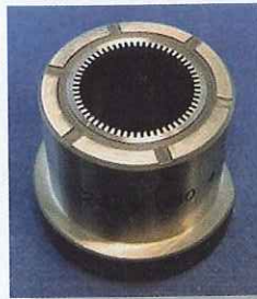
High precision fine tooth gear cavity insert
