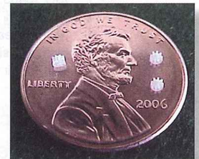
These 8 tooth spur gears are about the size of a grain of salt.
