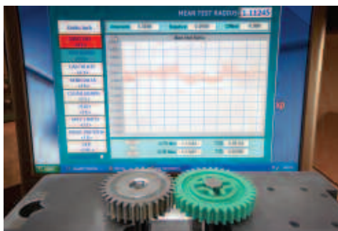
Double-flank rolling gear testers with certified master gears measure circular form and gear tooth accuracy.
